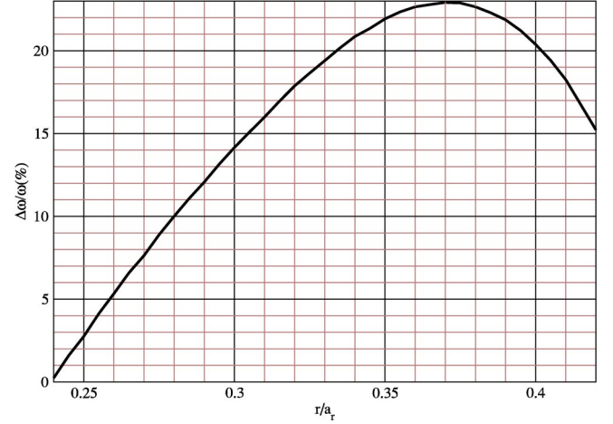
FIG. 19. The dependence of the relative size of the full photonic band gap as a function of the radius of the pores for a R_{2p}^{(1)} structure created using vertical pores drilling from 2D hcp lattices on perpendicular faces. a_r is the lattice constant of the hcp lattices.
